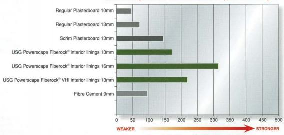
Impact Resistance for Cracking (joules)
